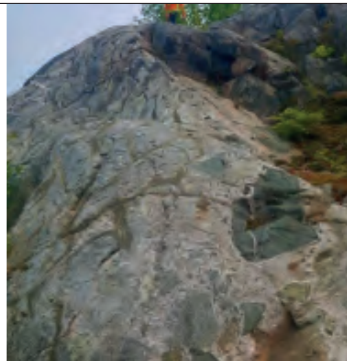
Figure 7-7 Brecciation and alteration associated with granite-metavolcanics contact
